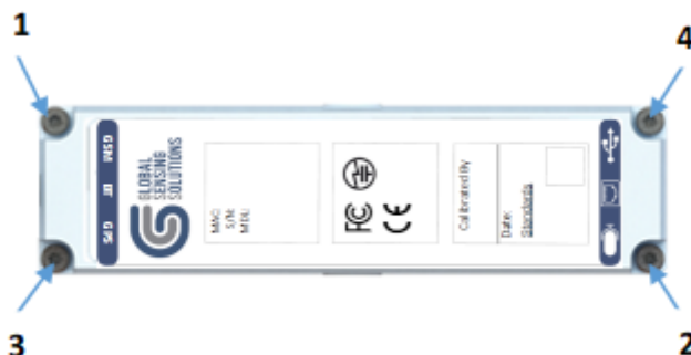
Figure 4 – Top Case Screw Removal Sequence
