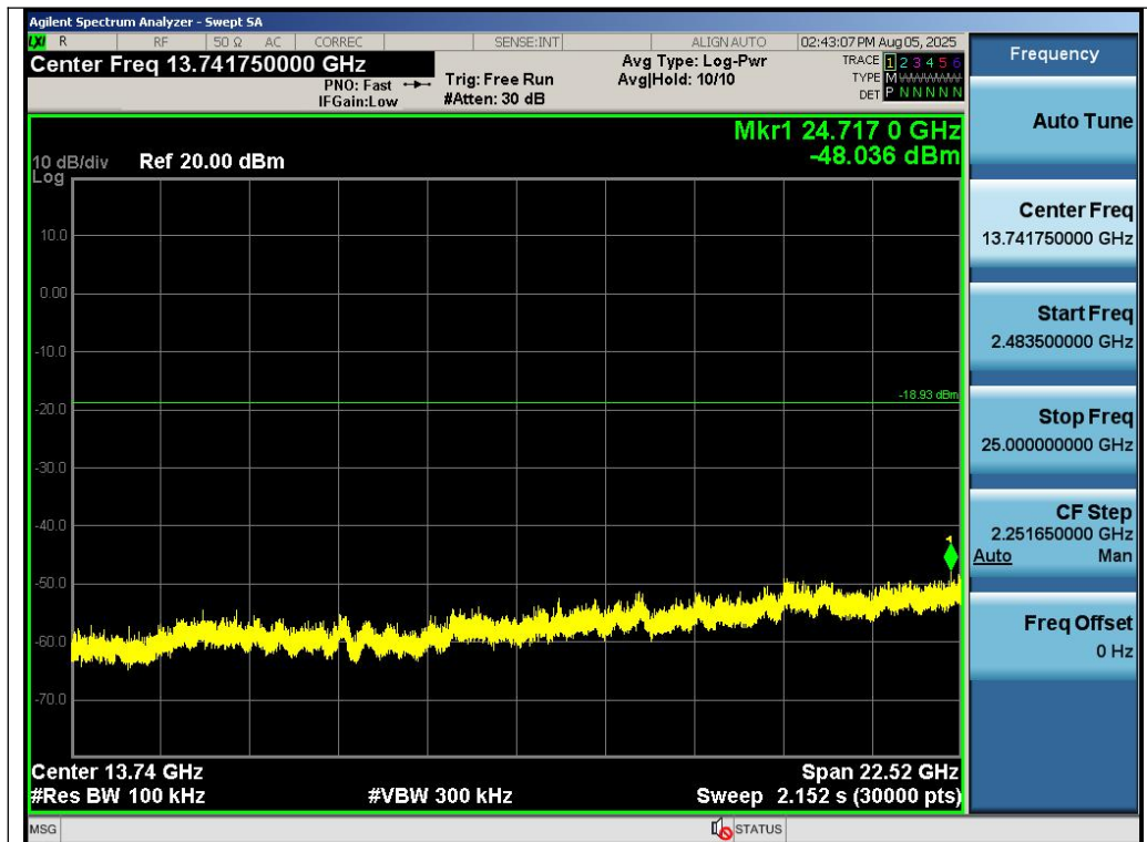
Test_Graph_LE2M_ANT1_2440_2Mbps_Higher Band Emissions
