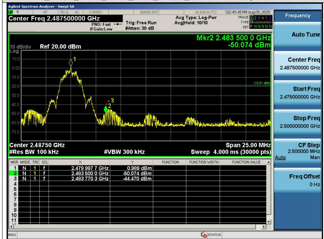
Test_Graph_LE2M_ANT1_2480_2Mbps_Higher Band Edge Emissions
