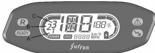
The power mode includes level 1, level 2, level 3, there will be corresponding number showing on the dashboard.
