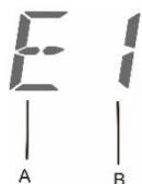
Note: Display one English letter in field A (Different English letters are displayed according to different feature modes). Display one number in field B (Different Numbers are displayed according to different feature levels).
