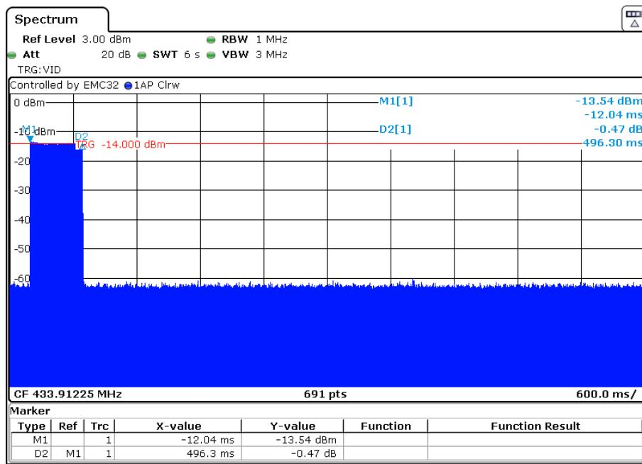
**3. Regulation 15.231 (a2)** A transmitter activated automatically shall cease transmission within 5 seconds after activation.
