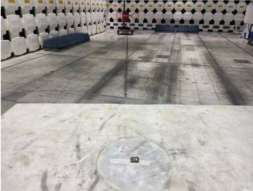
Radiated Emissions Test Setup (Worst-case axes), 30-1000 MHz
