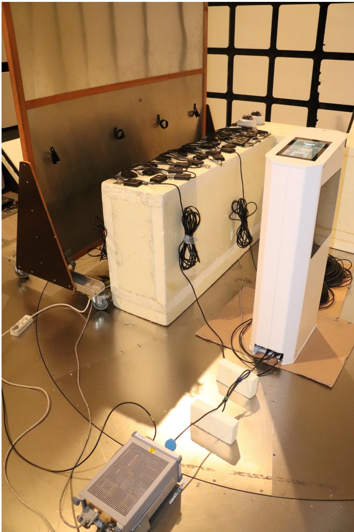
Photograph 1. Conducted emission setup
