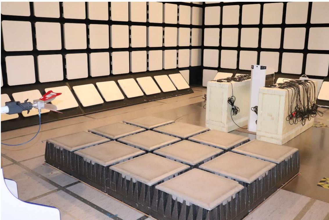
Photograph 3. Radiated emission test setup (1-18 GHz)
