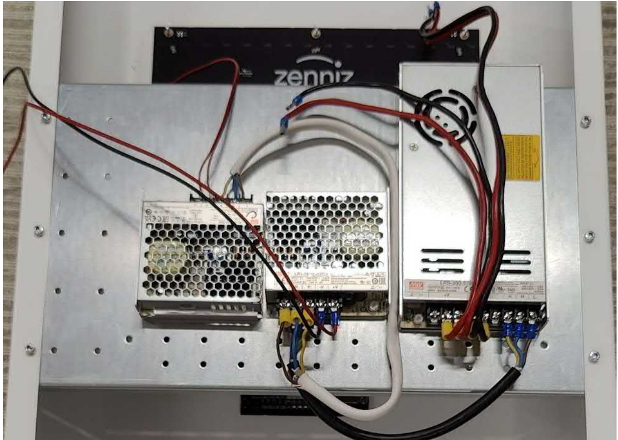
16. Connection of the powers for led panels, PoE and motherboard.
