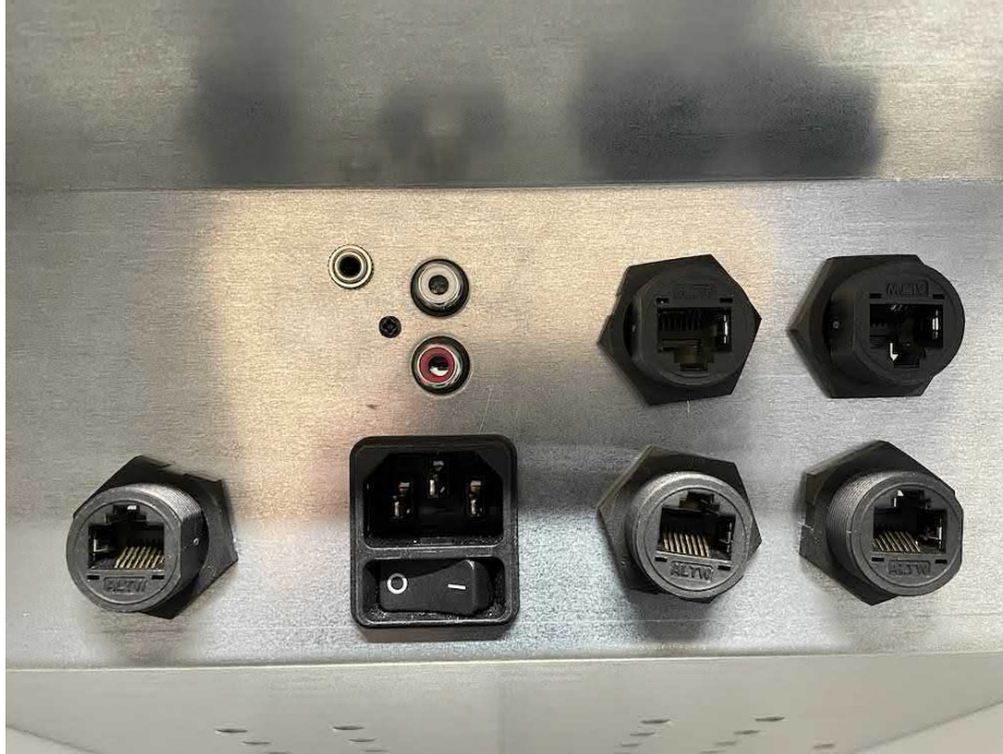
17. External ports. Top row from the left: Audio connectors, 2x RJ45 for the cameras Bottom row from the left: RJ45 for device, power, 2x RJ45 for the microphones
