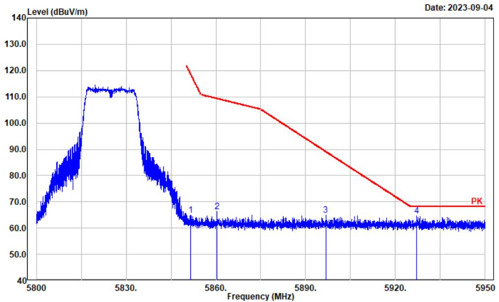
**Test plots for Radiated Spurious Emissions(802.11n ht20 5785MHz):
