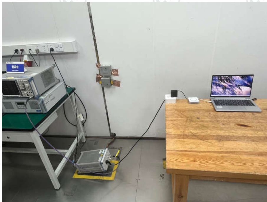
Conducted Emissions Test Setup
