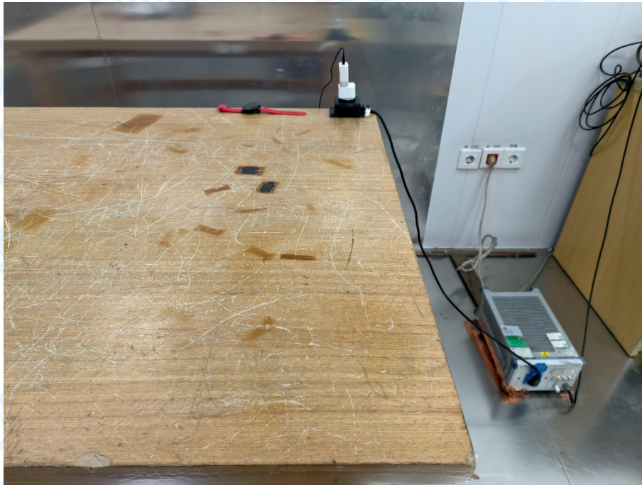
Photo of Setup for RF Conducted Emission
