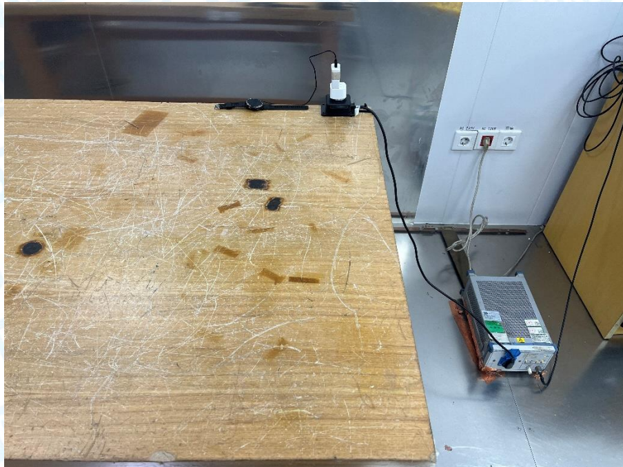
Photo of Setup for Radiated Emission (30MHz~1GHz)
