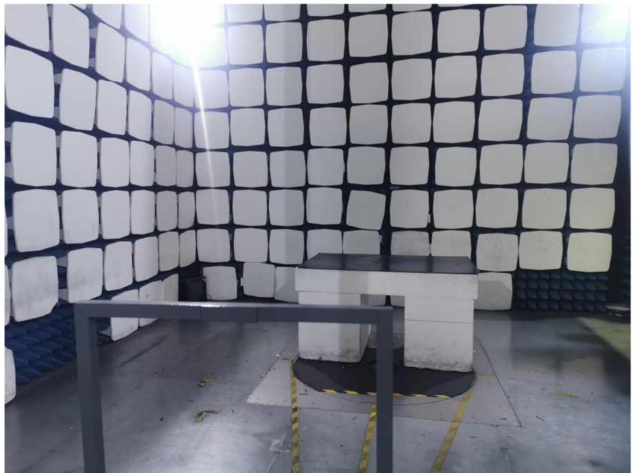
Radiation Emission Test Setup (Below 30MHz)
