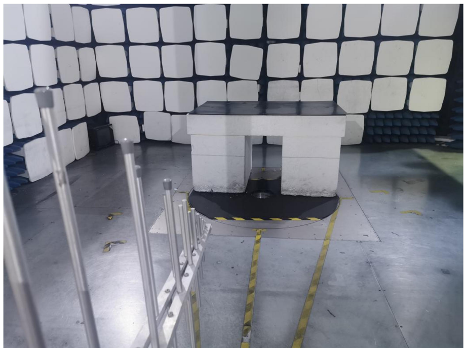
Radiation Emission Test Setup (30MHz to 1GHz)
