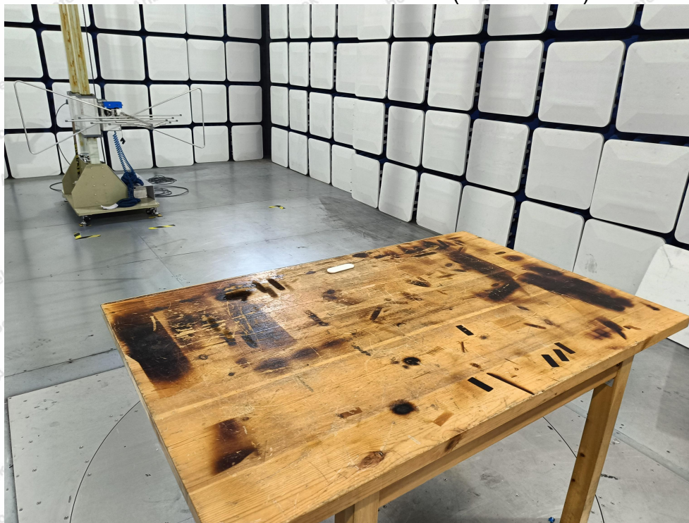
Photo of Radiation Emission Test (below 1GHz)
