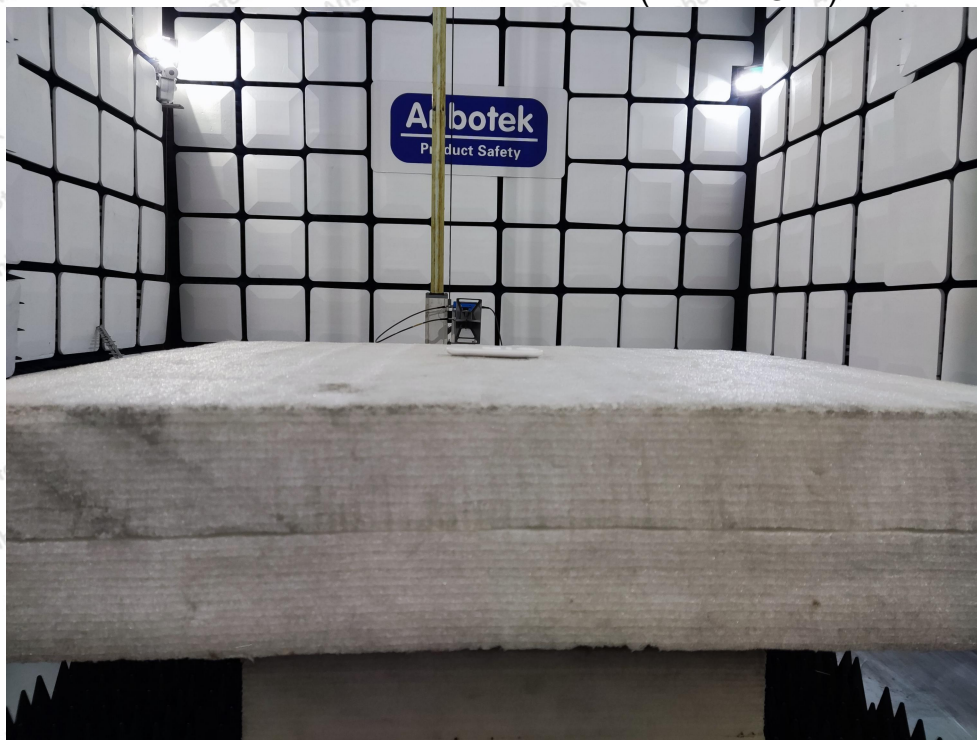
Photo of Radiation Emission Test (above 1GHz)
