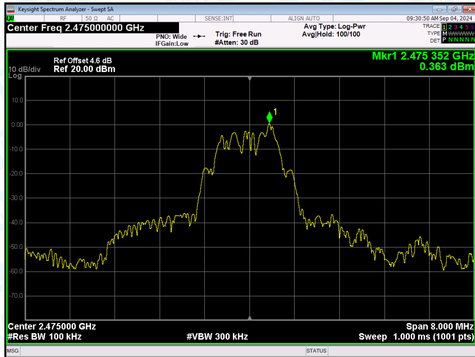
Band Edge NVNT 2475MHz Ant1 Emission
