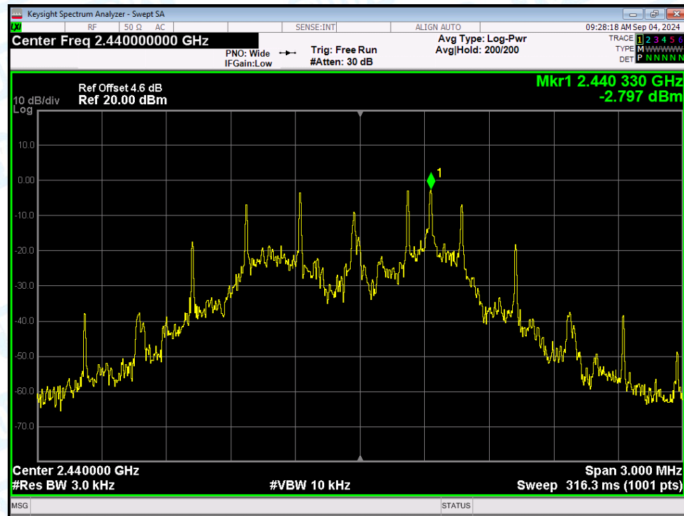
PSD NVNT 2440MHz Ant1
