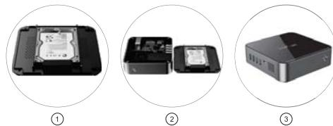
1. Remove the bottom cover of the machine and install the hard drive into the bay of the bottom cover.
