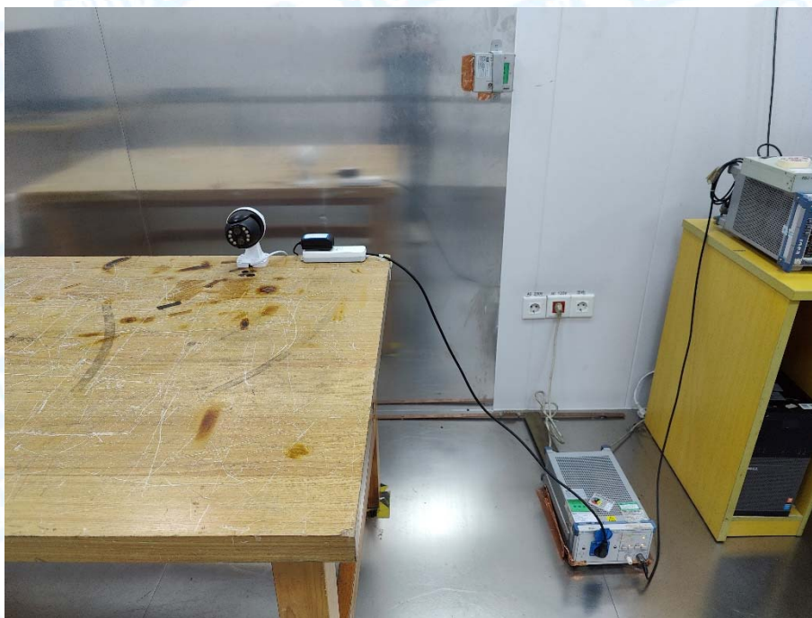
Photo of Setup for Conducted Emission
