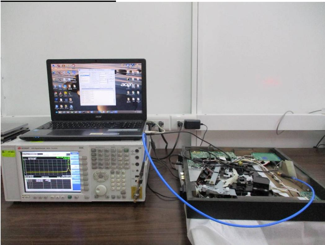
**CONDUCTED EMISSION MEASUREMENT SETUP****MODE: NORMAL OPERATION**
