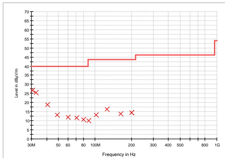
**CAQ450 HRV: 30 MHz to 1000 MHz, Vertical**
