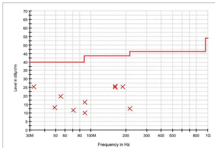
**CAQ350 HRV: 30 MHz to 1000 MHz, Vertical**
