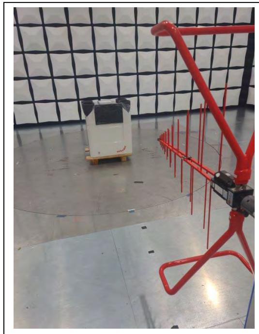
**CAQ450 HRV: Radiated Spurious Emissions Greater than 1 GHz**
