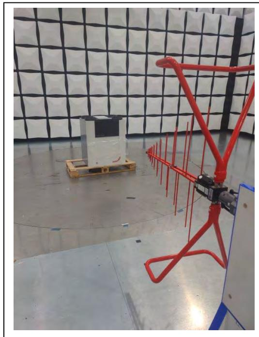
**CAQ600 HRV: Radiated Spurious Emissions Greater than 1 GHz**
