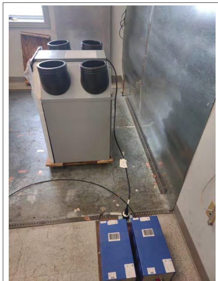
**CAQ350 HRV: Radiated Spurious Emissions Less Than 1 GHz**
