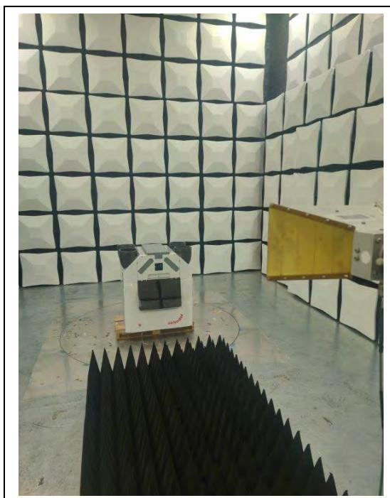
**CAQ450 HRV: Radiated Spurious Emissions Less Than 1 GHz**
