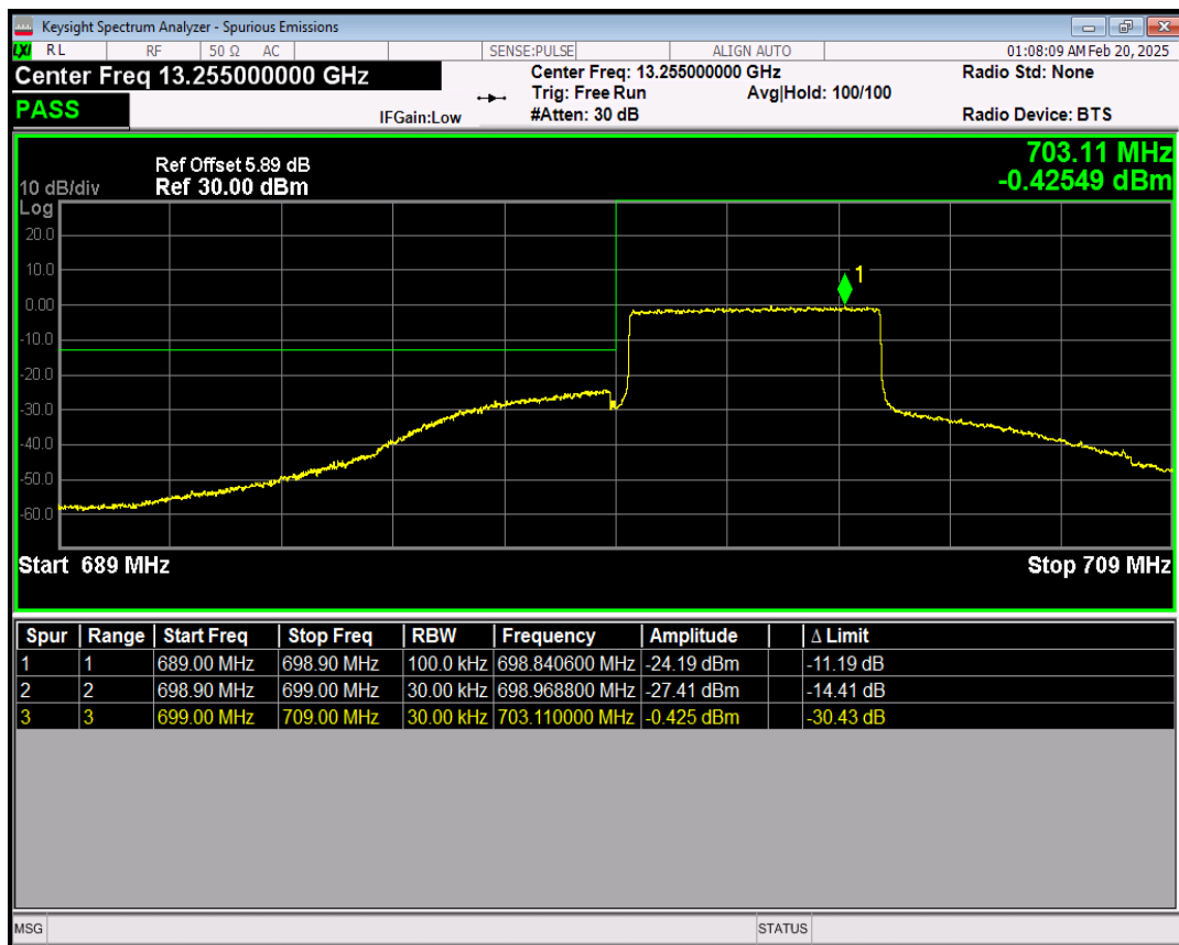
Band12 QPSK BW=5MHz Channel=23155 RB Size=1 Position=#0
