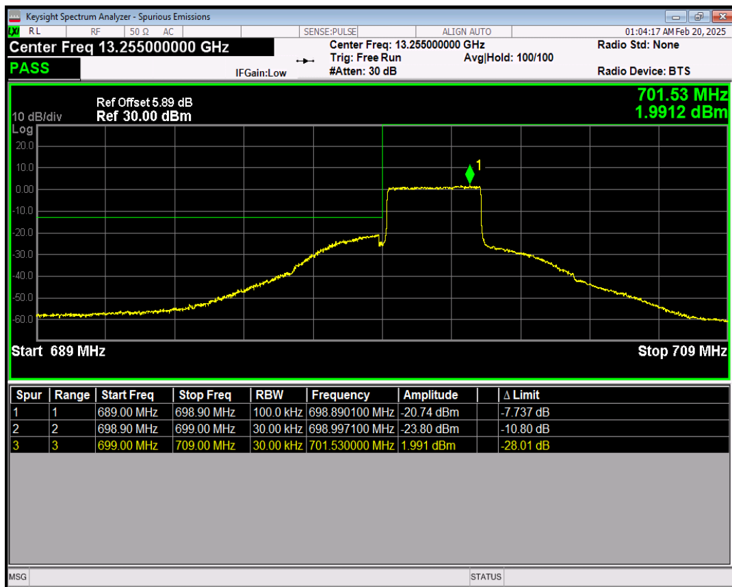
Band12 QPSK BW=3MHz Channel=23165 RB Size=1 Position=#0
