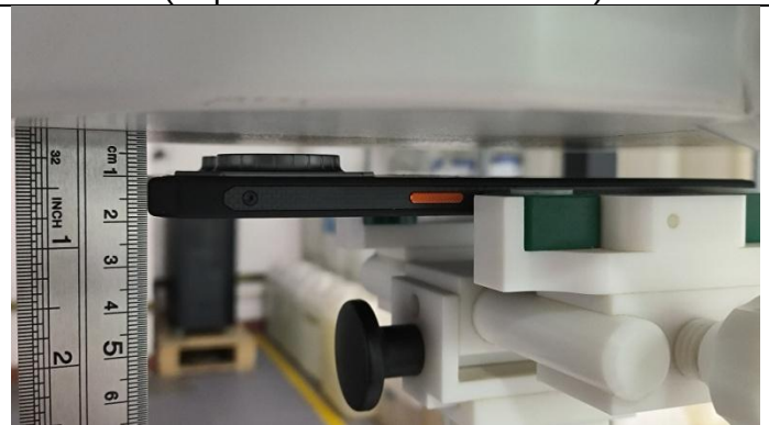
Right Side (Separation distance of 10mm)
