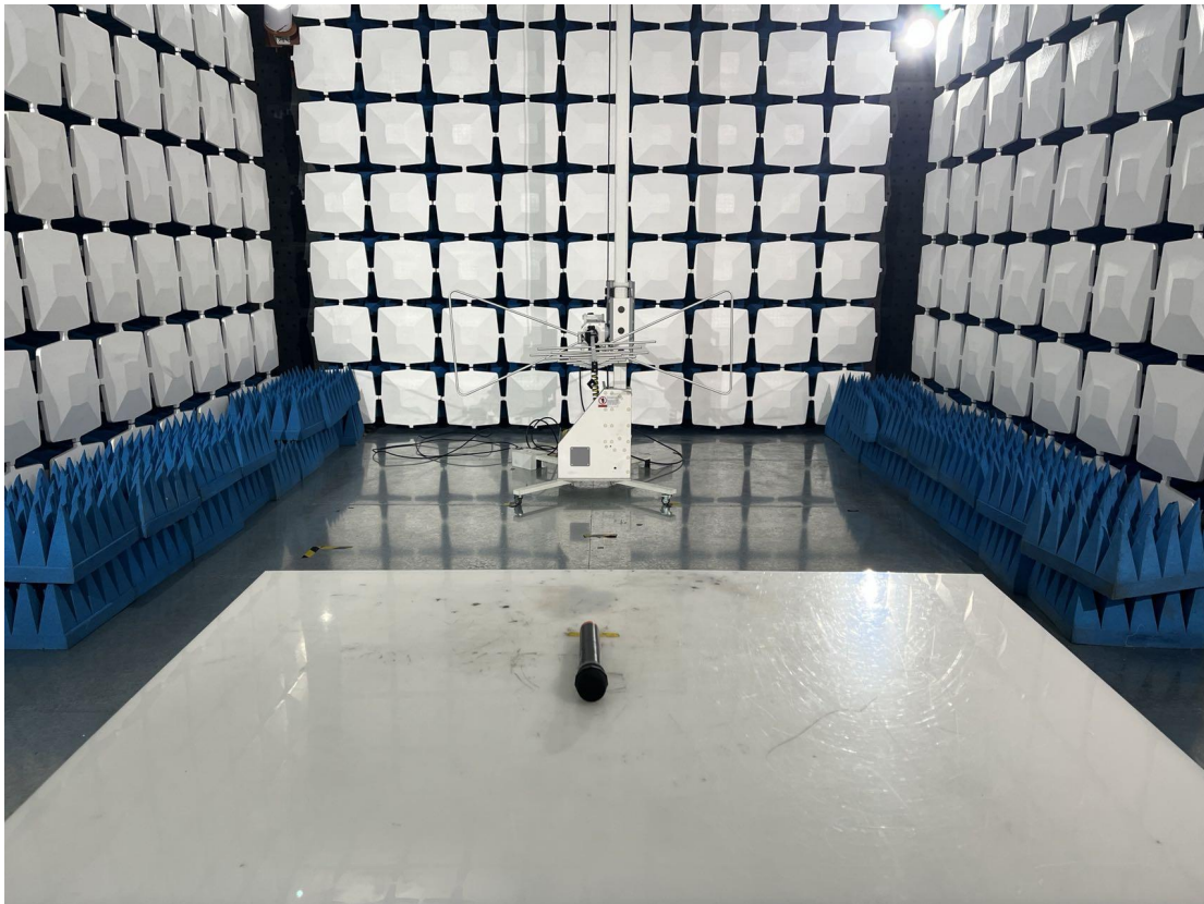
Above 1GHz for radiated emission test setup
