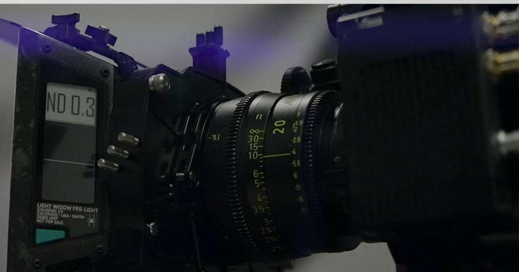
The tags are easily programmable using a phone app. Each filter tag can be programmed to include a custom display name, as well as different background colors and display modes.
