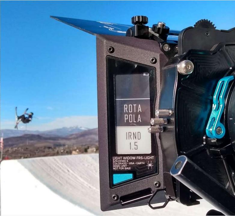
RFID stickers can also be added to self-contained filters such as rota-polas or diopters.
