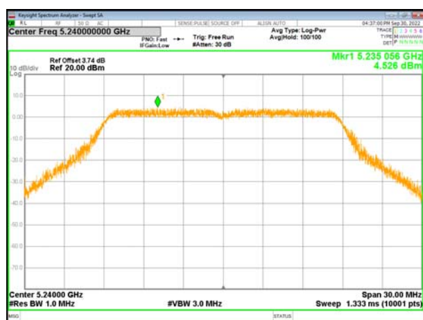
(802.11ac20) PSD plot on channel 48
