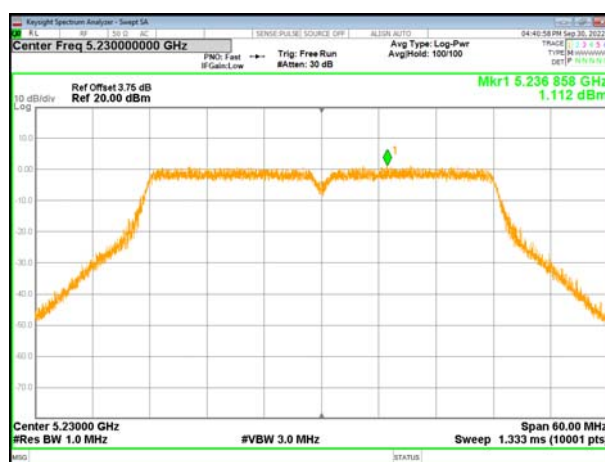
(802.11n40) PSD plot on channel 46
