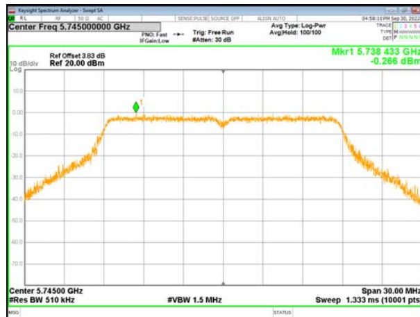
(802.11n20) PSD plot on channel 157
