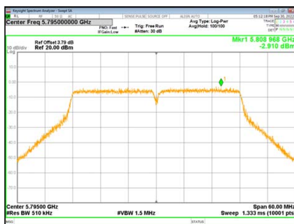
(802.11n40) PSD plot on channel 159
