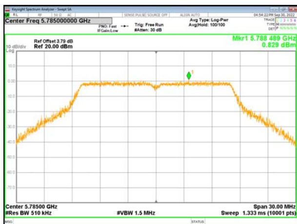
(802.11a) PSD plot on channel 165
