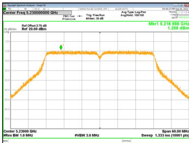
(802.11ac40) PSD plot on channel 46
