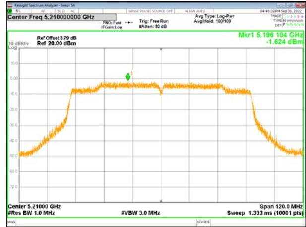
(802.11ac80) PSD plot on channel 42
