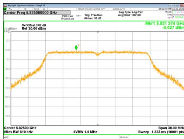
(802.11n20) PSD plot on channel 165
