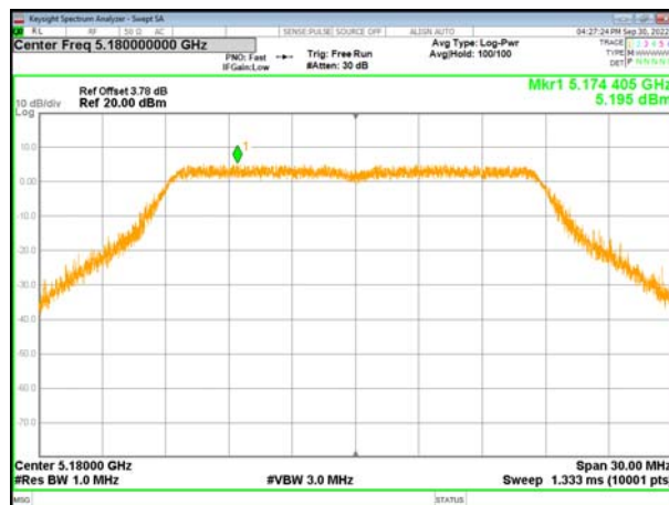
(802.11n20) PSD plot on channel 40
