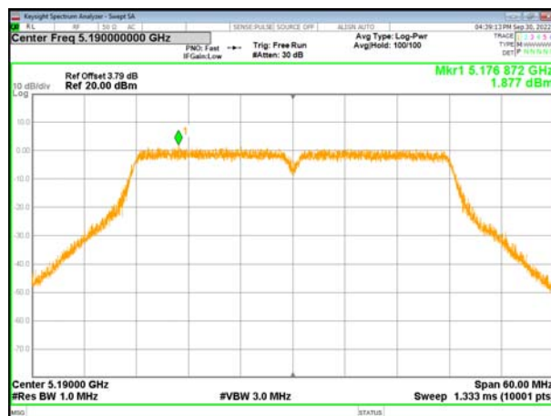
(802.11n40) PSD plot on channel 38
