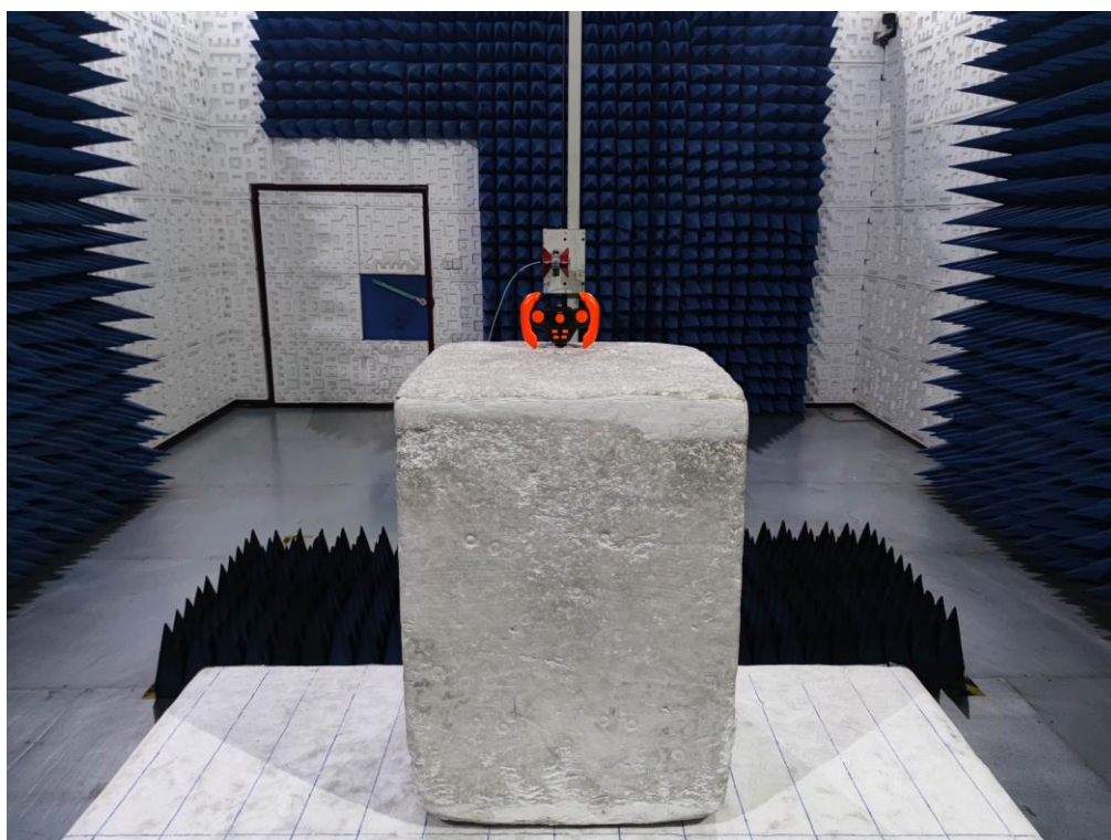
RADIATED EMISSION TEST SETUP ABOVE 1GHz
