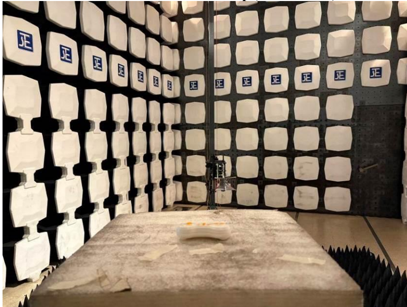
Radiated emissions test set up (Above 1GHz)
