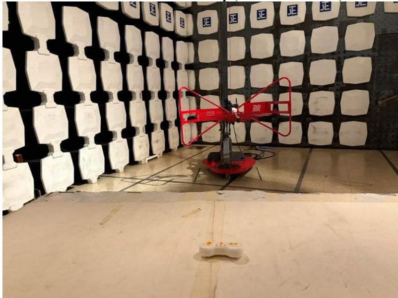
Radiated emissions test set up (30MHz-1000MHz)
