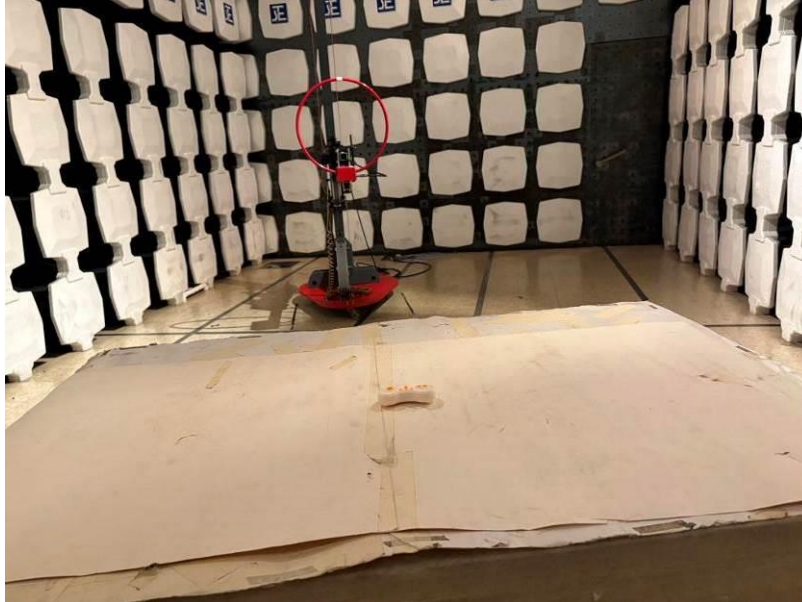
Radiated emissions test set up (9KHz-30MHz)
