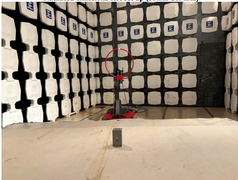
Radiated emissions test set up (9KHz-30MHz)
