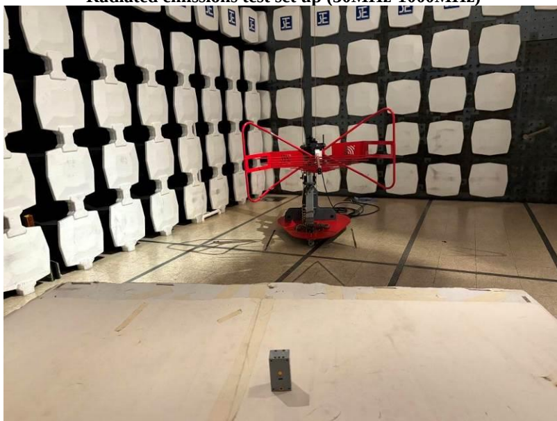
Radiated emissions test set up (30MHz-1000MHz)
