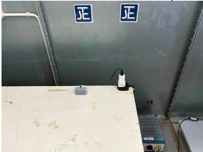
Measurement of Conducted Emission Test Set Up
