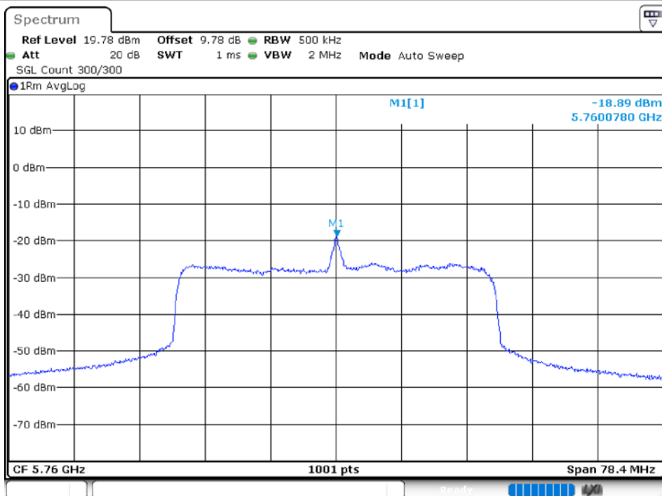
PSD NVNT 40M 5820MHz Ant 2
