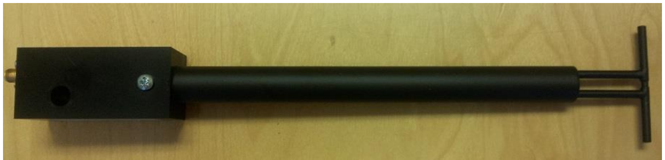
Figure 1 – MVG COMOSAR Validation Dipole
