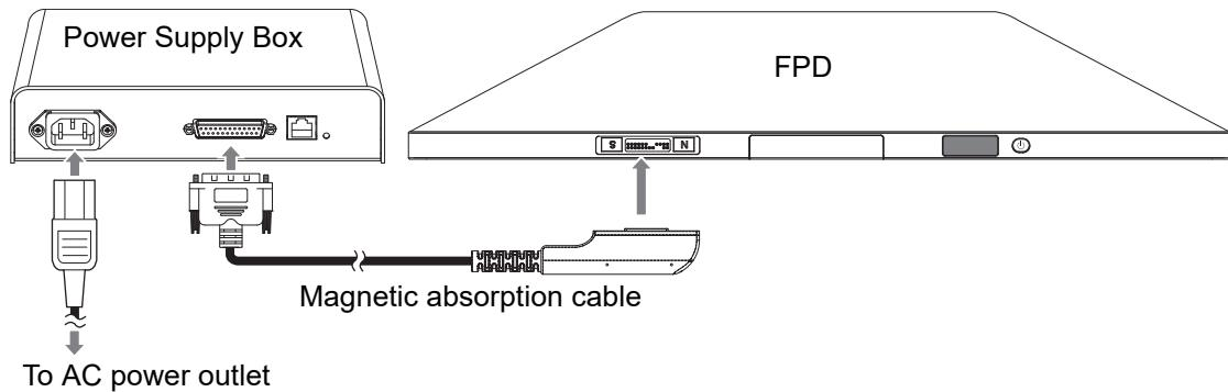
1. Connect the FPD to the Power Supply Box using the magnetic absorption cable.
