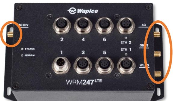
In case the device needs to be connected via one of the above wireless interfaces, the specific antennas must be connected to the device. Wapice may offer them upon request. No warranty is given, and no responsibility taken for defects of the third-party items offered by Wapice. The recommended tightening torque for the SMA connectors of the device is 0,4 Nm. Unused antenna connectors shall be fitted with a protective cap to ensure IP65 water protection.
