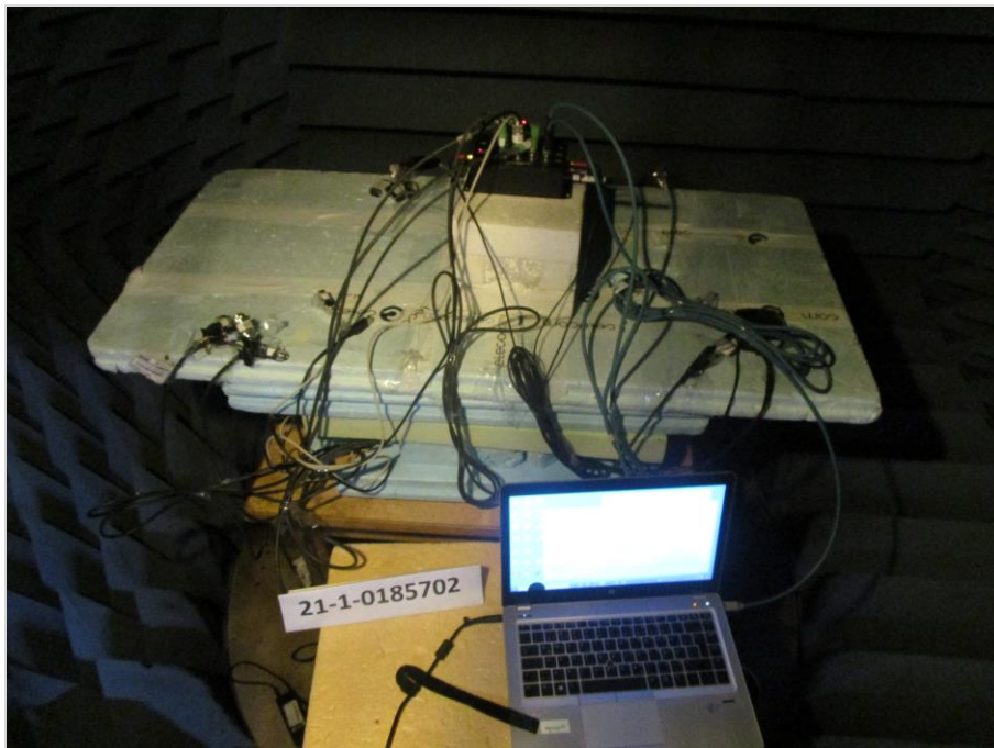
Photograph 3: EUT test setup in the fully anechoic chamber°
