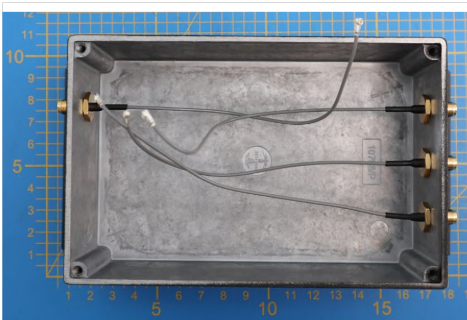
Photograph 3: bottom side of enclosure with antenna connectors inside view
