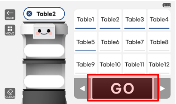
④ Touch the 'GO' button and the robot will start serving in that position.
