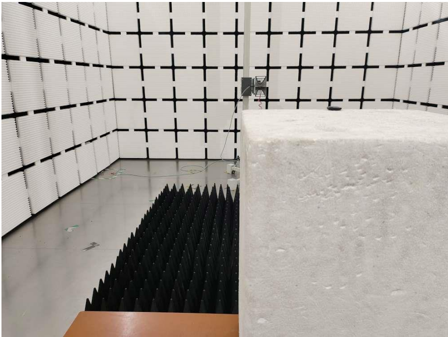
Radiated Emission Test View Above 1GHz
