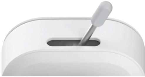
2. Holding the Emitter by its handle, slide the Emitter cleat downward into the Wireless Charger's matching holstering wings until it settles into position.
