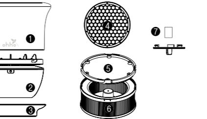
① Upper case ② Lower Parts ③ Charging Dish ④ Main Filter
