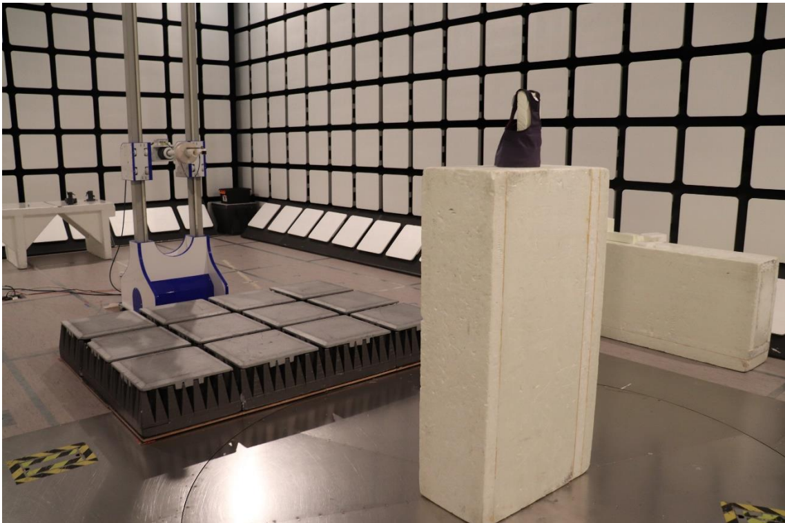
Photograph 6. Test setup for Radiated emissions (18 – 25 GHz)
