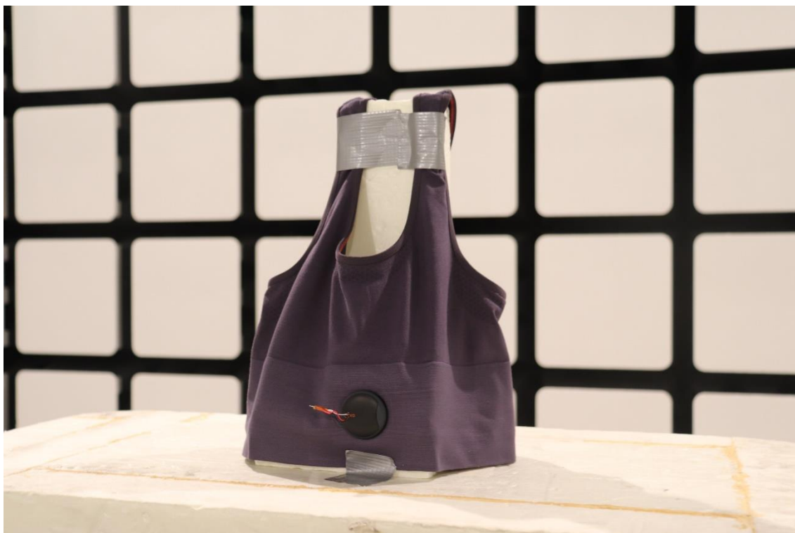
Photograph 2. The EUT orientation during Radiated emissions
