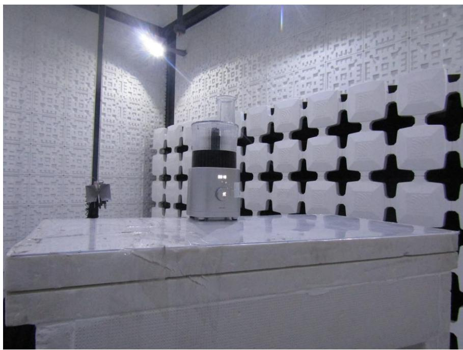
Conducted disturbance voltage at mains ports (150KHz-30MHz)
