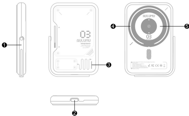
1. Metal foldable kickstand, can be unfolded to hold the phone.
