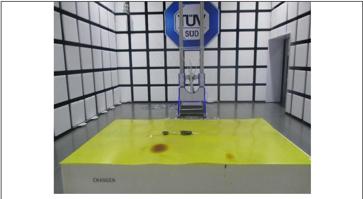
Details of: Radiated Emission test (above 1GHz)
