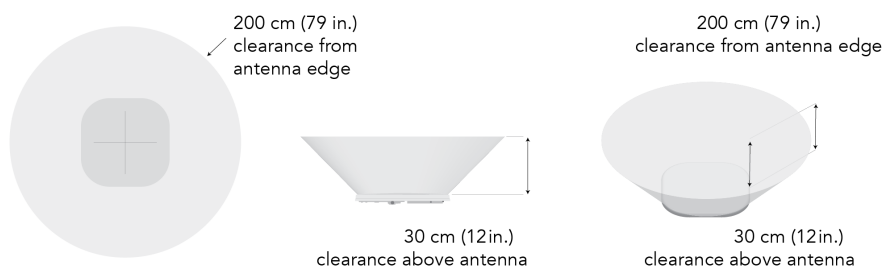
Figure 3: Keep out region (gray cone) and safe region (outside the gray cone) for the 40 W UT, designated for occupational use
