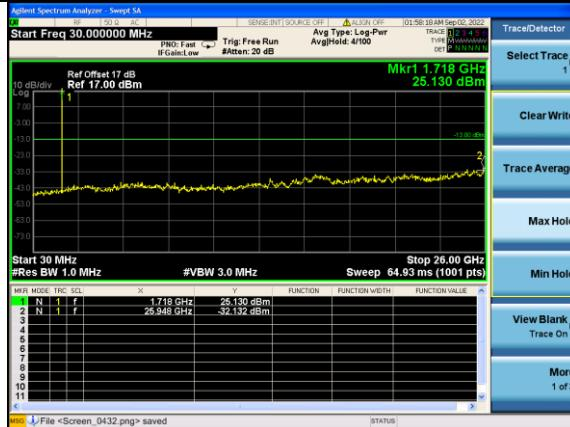
Test Mode: LTE Band 4 / 1.4MHz /6RB
