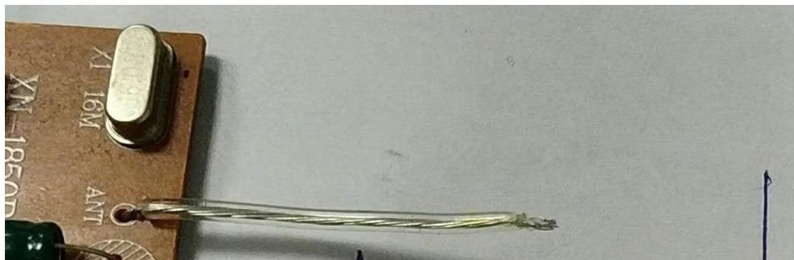
Note: The 2.4G transparent antenna specification is 9-core 1.3mm outer diameter tinned copper wire, transparent color, length of 40mm, wire end stripped 3MM and tinned. Compliant with environmental standards: EU EN71 (19E), ROHS, PAHS, 6P~16P, European and American CPSIA, HR4040.
