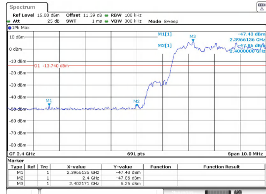
Out Of Band Emission(Left) \pi/4 DQPSK_2-DH5_Channel Hopping
