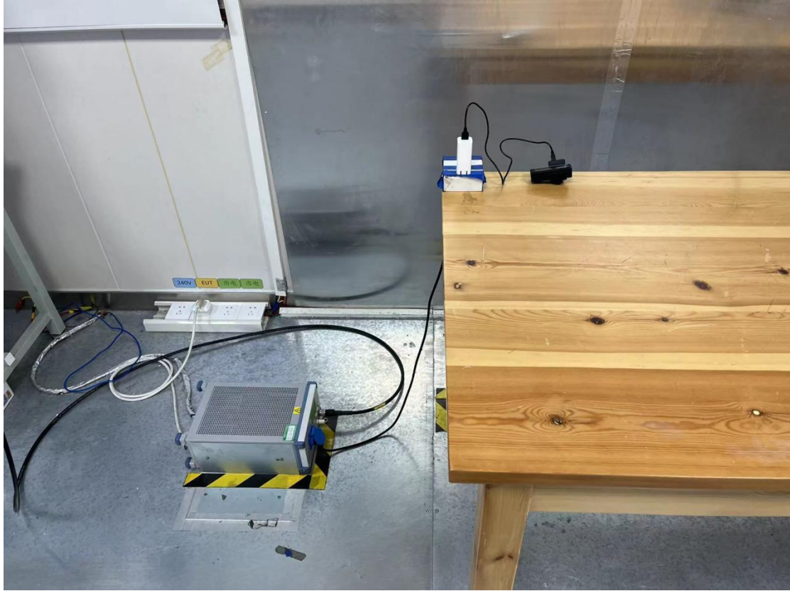
Conducted emission test setup
