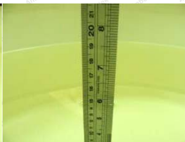
Photo of Liquid Height for Body SAR
