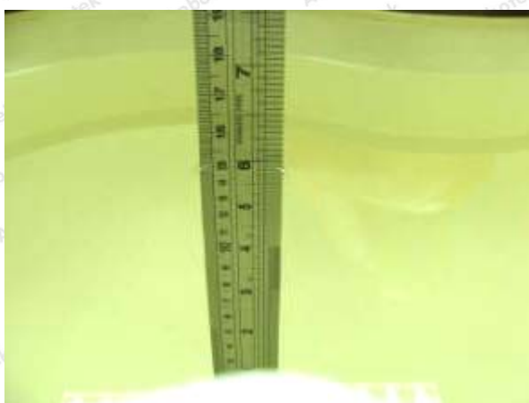
Photo of Liquid Height for Head SAR
