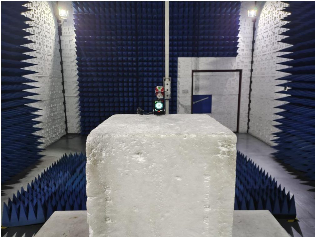
RADIATED EMISSION TEST SETUP ABOVE 1GHz
