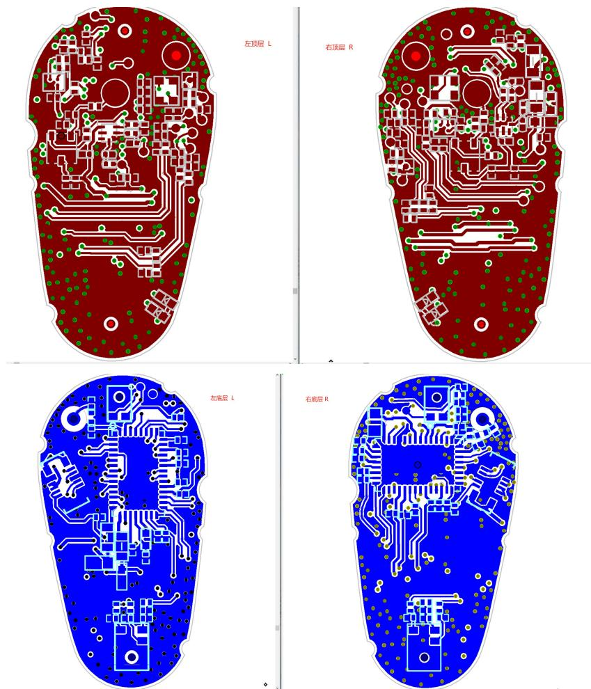
Hydrabuds (AH150) is wireless Bluetooth TWS earphones, a pair of earphones are divided into left and right earphones, the appearance is different, but the internal PCBA circuits are the same. It's because the earphone structure is not mirrored, resulting in PCBA appearance differences.
