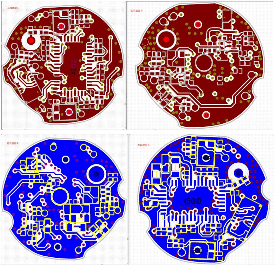
Hydrabuds (AH148) is wireless Bluetooth TWS earphones, a pair of earphones are divided into left and right earphones, the appearance is different, but the internal PCBA circuits are the same. It's because the earphone structure is not mirrored, resulting in PCBA appearance differences.
