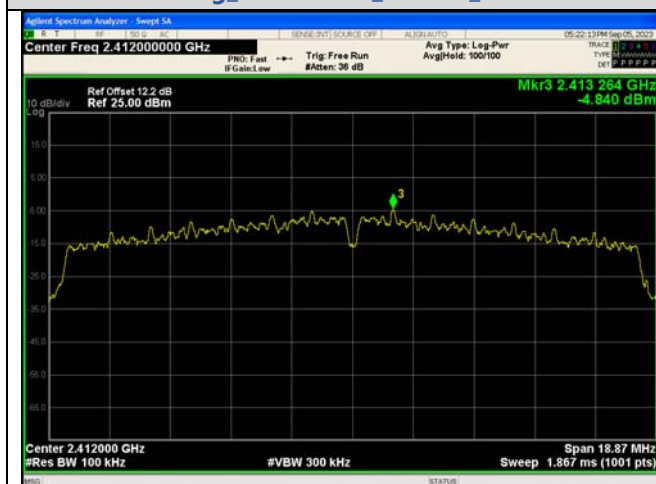
In-Band Reference Level IEEE 802.11n_Channel 1_20MHz_Antenna 0
