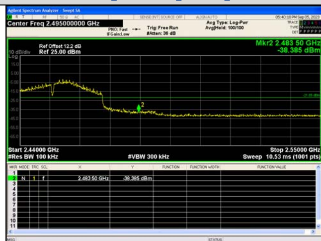
Out Of Band Emission IEEE 802.11n_Channel 9_40MHz_Antenna 0
