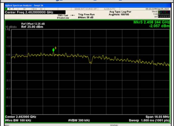
In-Band Reference Level IEEE 802.11g_Channel 11_20MHz_Antenna 0
