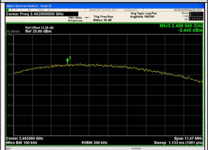
In-Band Reference Level IEEE 802.11b_Channel 11_20MHz_Antenna 0
