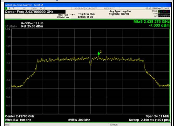
In-Band Reference Level IEEE 802.11g_Channel 6_20MHz_Antenna 0
