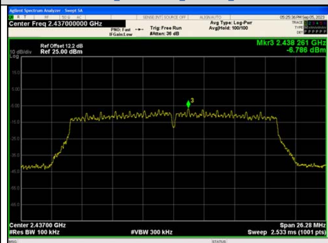
In-Band Reference Level IEEE 802.11n_Channel 6_20MHz_Antenna 0
