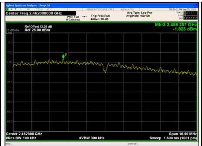
In-Band Reference Level IEEE 802.11n_Channel 11_20MHz_Antenna 0
