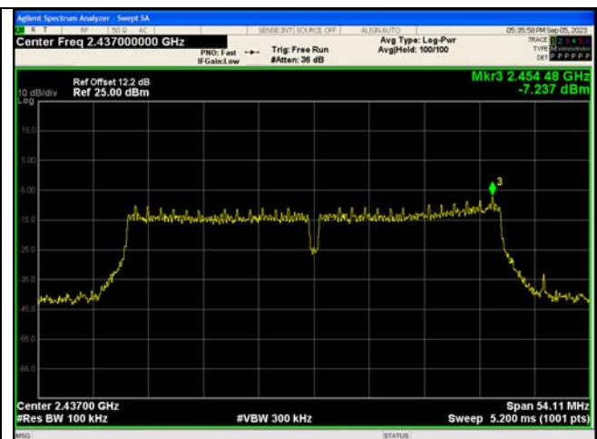
In-Band Reference Level IEEE 802.11n_Channel 6_40MHz_Antenna 0
